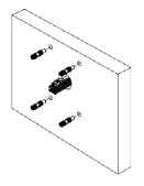
2. The safety wire has 2 hooks at both sides. Hook the safety wire(A) on the wall mount and pull the cable through the wall mount and fasten screws to secure the wall mount on the wall.
