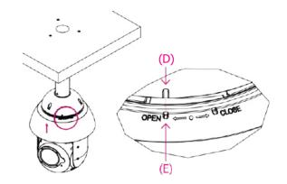
6. Follow the CLOSE direction to rotate tightly the camera and then tighten screws (3pcs) to fix the camera on the CAP.
