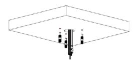
2. Pull the safety wire and cables through the bottom case of pendant mount and tighten the screws.
