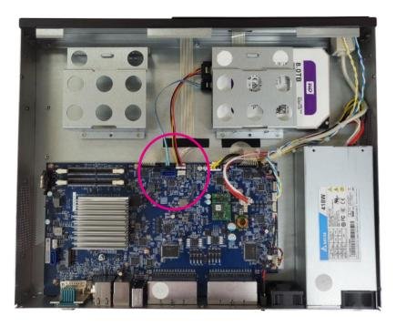
4. Remove the HDD bracket (Left).
