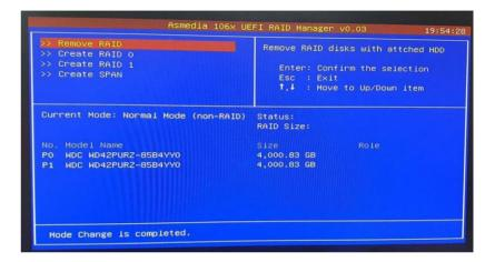
The main menu allows you to select from several setup functions. Use arrow keys to select among the items and press to "enter" to select the function.
