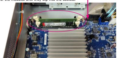
3. Release the locks on the second DIMM memory sockets. Insert the other module into the sockets also at a 90 degree angle. Apply firm even pressure to each end of the modules until they slip into the sockets.
