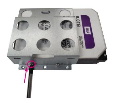
3. Plug in the HDD SATA cable\*\* and SATA power cable\*, lock the screw into the system.
