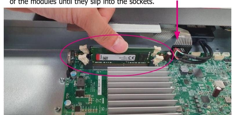
2. Release the locks on the second DIMM memory sockets. Insert the other module into the sockets also at a 90 degree angle. Apply firm even pressure to each end of the modules until they slip into the sockets.
