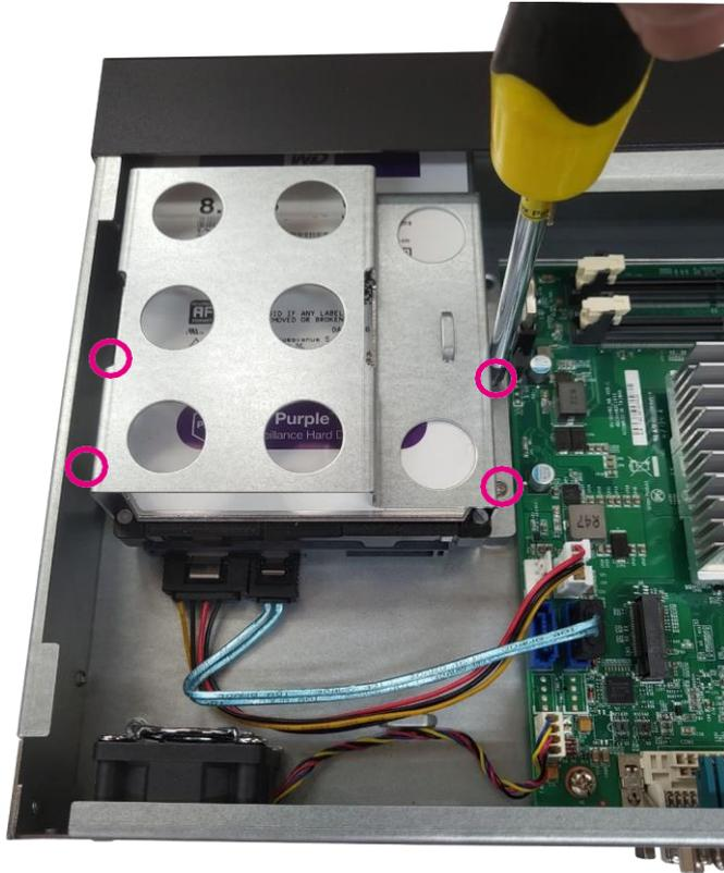
5. Tightening Cable Guidance For 3.5" HDD
